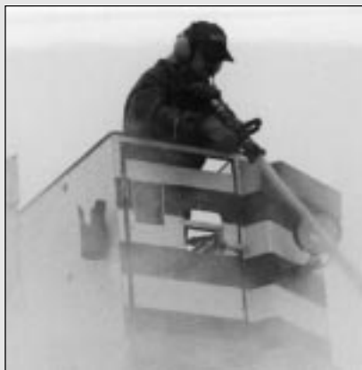
Hot water under pressure in a tight stream was required to break ice free from an aircraft wing.
