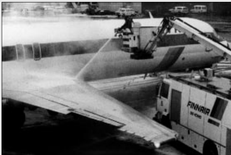
Ice forms more readily over the wing root, where the cold fuel settles and there is more metal structure, including the landing gear components, which can contribute to colder temperatures.
