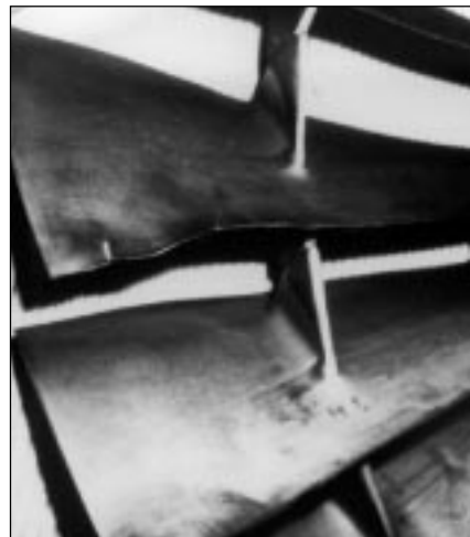
The gentle bend in the blades is characteristic of soft foreign object damage.
